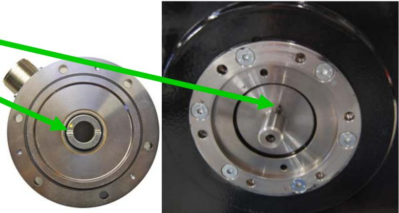
2. The cable output of the encoder housing must show in the direction of the terminal box of the vibration drive.
