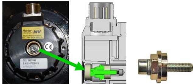
4. Attach encoder by means of hexagonal screws and Nordlock lock washers. Fix screw cap to the encoder.
